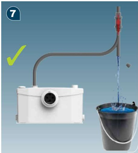
Wye fitting on the discharge line to facilitate drainage of vertical pipe.
